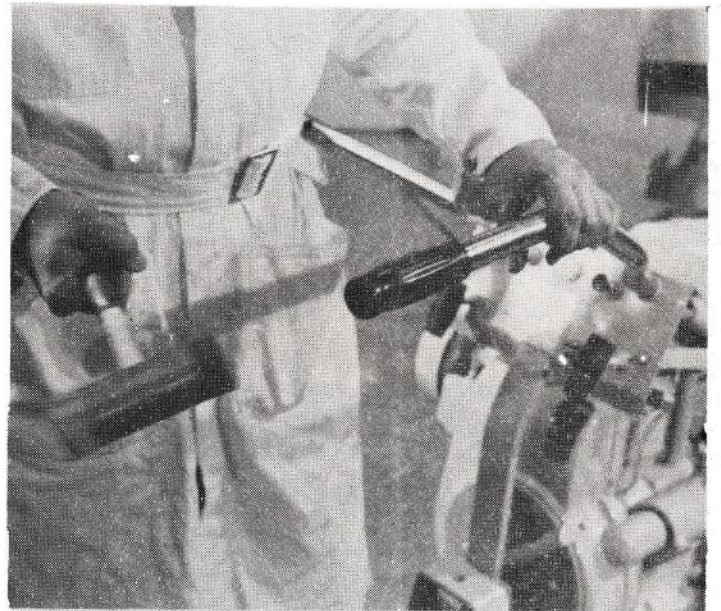
15. Wet inside of Handle Grips with clean water only (DO NOT use oil or soap). Start Handle Grips on Handle Bars. Drive the Grips on with a soft mallet.
