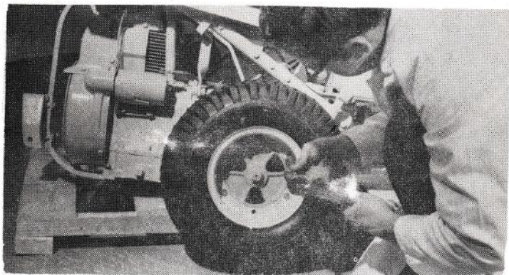
6. Install Wheel Assembly on Right Hand Wheel Hub. Valve Stem to outside.
