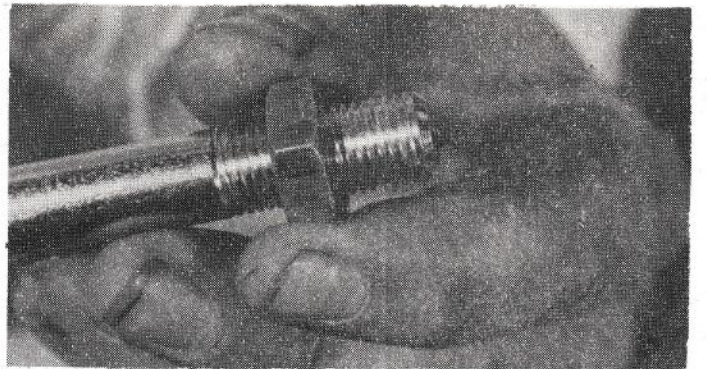
16. Thread Jam Nut on long threaded end of Shifter Rods.
