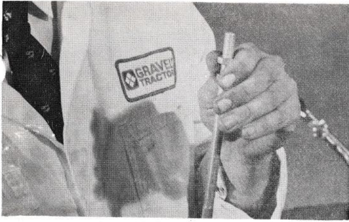
23. Thread TWO Jam Nuts on each Clutch Rod, approximately 6 inches from end.
